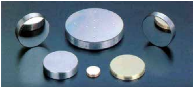
STANDARD BLOCKS FOR HARDNESS 생산 item은 Rockwell, Rockwell Superficial, Shore, Vickers, Micro Vickers, Brinell 등 Product items include Rockwell Superficial, Shore, Vickers, Micro Vickers, and Brinell
